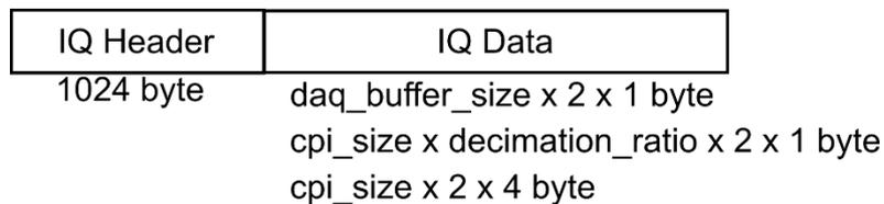
Figure 1: IQ Data frame structure
